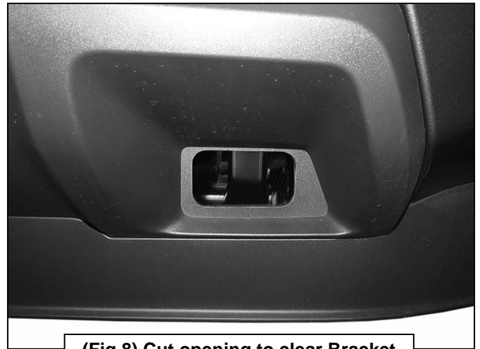
(Fig 8) Cut opening to clear Bracket
