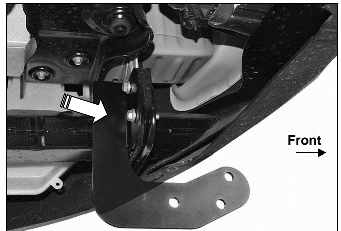
(Fig 6B) Use 12mm x 32mm Large Flat Washer for a spacer on lower mounting bolt only between Mounting Bracket and bumper bracket (Driver side Bracket installation pictured)
