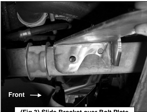
(Fig 3) Slide Bracket over Bolt Plate
