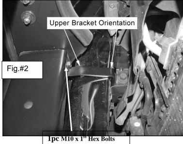
2pcs 10mm Oversized Flat Washer 1pc 10mm Lock Washer 1pc M10 Hex Nuts
