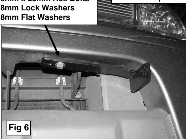
05-08 driver side Top Bracket installation pictured
