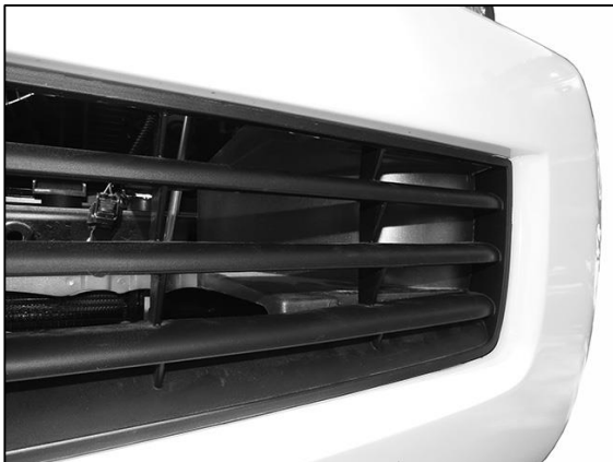
(Fig 5A) Remove or cut air deflector from behind lower grille opening in bumper
