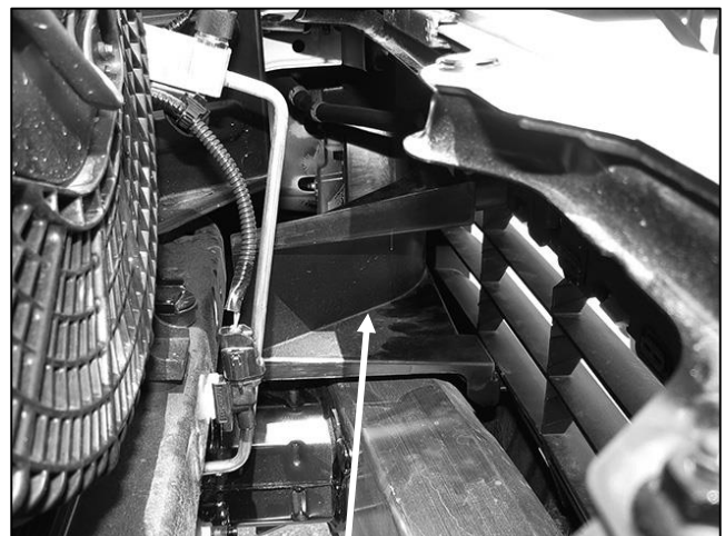
(Fig 5B) Air deflector on driver side pictured from behind bumper. Note: Not included on all models
