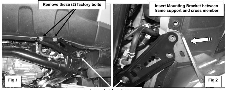
Loosen but do not remove this factory bolt if needed
