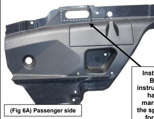
Install and align the Bull Bar as per instructions, tighten all hardware before marking the area on the splash guard to cut for clearance. Cut along dotted line.
