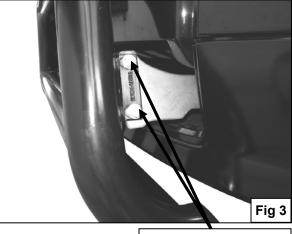
10mm x 35mm Hex Bolts 10mm Lock Washers 10mm Flat Washers 10mm Hex Nuts
