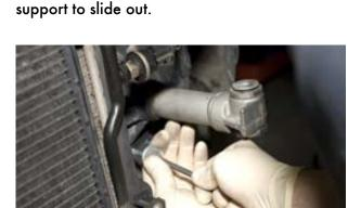
10. Temporarily re-install the longer front bumper strut bolts (1 on each side). This will allow the core
