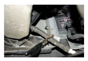
**6.** Disconnect intake funnel from the top of the air box to allow the core support to move.
