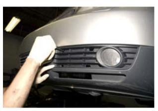
\* 1.8T B6 and 2.0T B7 does not require the removal of the bumper/core support. The snub mount can be removed by loosening the 3 - 6mm allen bolts and then remove/replace the snub mount bracket assembly. Torque those 3 allen bolts to 19ft lbs.\*
