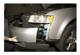
**7.** Remove 4 fender screws from core support (2 on each side) with a T30 Torx.
