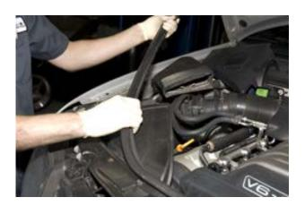
9. Remove 6 bumper strut bolts (3 on each side) using a T45 Torx.
