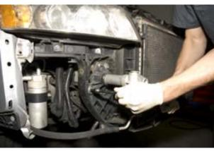
11. Pull core support away from the engine to allow workspace. Remove old snub mount (may be broken as pictured below).
