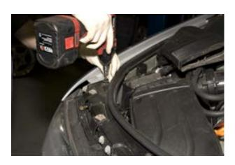
**4.** Disconnect fog light wiring, disconnect and clamp headlight washer nozzle line. Loosen 4 bumper bolts with 10mm socket. Remove lower valence screws from fender liner with T25 torx
