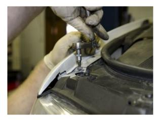
10. Re install the snub mount engine bracket and tighten the 3 13mm bolts, torque them to 37ft lbs. Reinstallation of all parts is reverse of removal, and Torque values are as follows:
