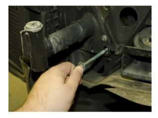
9. Back underneath the car, push the BFI performance Snub Mount into place – pay close attention to face the rounded edge side of the mount towards the front of the car when placing on the mount stanton. This will be difficult and we recomend using a slight amount of grease to make install easier.
