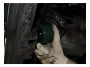
8. Remove the 4 T30 bolts from the top of the lock carrier as well as the two T30 bolts beneath the headlights on the fender. Pull the lock carrier away from the car several inches to allow room for the snub mount to be installed.
