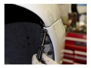
**6.** Using the T45 Torx bit, remove the six crash support bolts (three on each side)to loosen the lock carrier.
