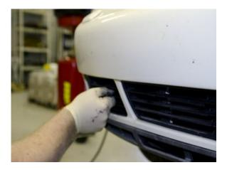
**3.** Using the 6mm Allen key socket, remove the two bumper bolts (located inside the grille opening, that run vertically through the bumper rebar.
