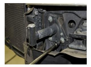
7. Thread in the bumper bolts to one of the crash support holes on each side. You will use these bolts to slide the lock carrier to the service position
