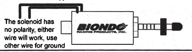
When hooking up this solenoid to our Mega Series delay box or one of Biondo shift boxes, follow this diagram.
