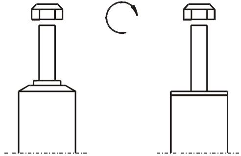
**Do not use an impact tool to loosen or tighten fasteners due to possible damage to the product.
