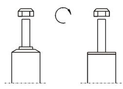
Do not use an impact tool to loosen or tighten fasteners due to possible damage to the product. Self- locking nuts must only be used once!
