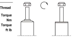
Do not use an impact tool to loosen or tighten fasteners due to possible damage to the product. Self- locking nuts must only be <u>used once</u>!
