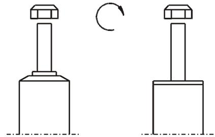
**Do not use impact tools for loosening or tightening fasteners, because this may destroy the threads. Self- locking nuts must only be used once!**
