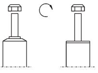
DO NOT USE IMPACT TOOLS FOR LOOSENING OR TIGHTENING FASTENERS, BECAUSE THIS MAY DESTROY THE THREADS. SELF- LOCKING NUTS MUST ONLY BE <u>USED ONCE</u>!
