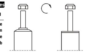
Do not use an impact tool to loosen or tighten fasteners due to possible damage to the product. Self- locking nuts must only be <u>used once</u>!
