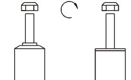
Do not use an impact tool to loosen or tighten fasteners due to possible damage to the product. Self- locking nuts must only be used once!
