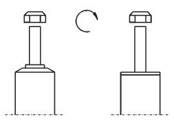
Do not use an impact tool to loosen or tighten fasteners due to possible demage to the product.
