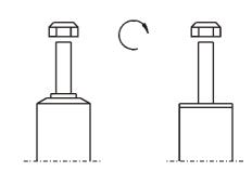
DO NOT USE IMPACT TOOLS FOR LOOSENING OR TIGHTENING FASTENERS, BECAUSE THIS MAY DESTROY THE THREADS. SELF- LOCKING NUTS MUST ONLY BE USED ONCE!
