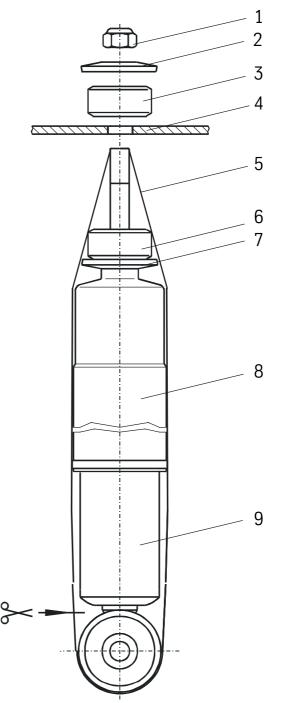
Do not remove fixing strap before fitting BILSTEIN shock absorber, it is to be use for mounting aid!
