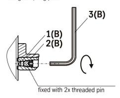
Fix the spring plate with the rubber pins/ balls (1) and set screw (2) by using the auxiliary tool (hex key (3)).
