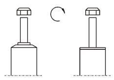
Do not use an impact tool to loosen or tighten fasteners due to possible damage to the product. Self- locking nuts must only be <u>used once!</u>
