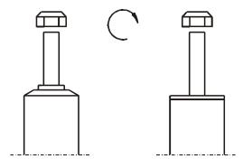
Do not use an impact tool to loosen or tighten fasteners due to possible demage to the product. Self- locking nuts must only be used once!
