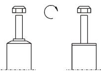
Do not use impact tools for loosening or tightening fasteners, because this may destroy the threads. Self-locking nuts must only be used once!
