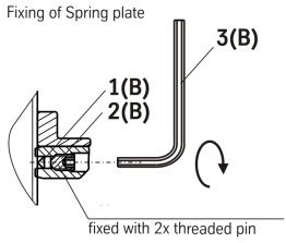
Fix the spring plate with the rubber pins/ balls (1) and set screw (2) by using the auxiliary tool (hex key (3)).
