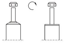
Do not use impact tools for loosening or tightening fasteners, because this may destroy the threads. Self- locking nuts must only be <u>used once!</u>
