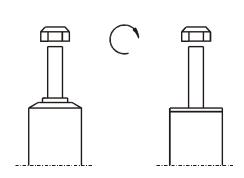
Do not use an impact tool to loosen or tighten fasteners due to possible damage to the product.
