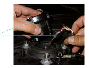
Remove nuts on suspension strut tower
