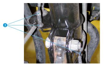
Disconnect coupling rod from suspension strut 4
