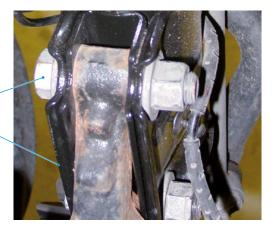
Where applicable, remove balance weight on top of strut and disconnect shock absorber plugs 6
