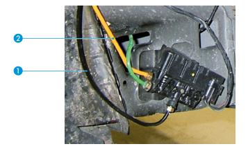
Detach brake hose, ABS cable and (if necessary) electrical line of the brake pad wear sensor from suspension strut. 3
