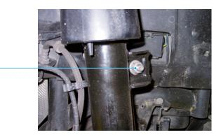
Remove nuts and bolts from suspension strut mounting on axle leg (5)
