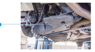
Disassemble the connection to the height sensor (9) at the traverse link
