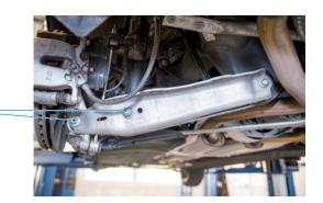
Secure the air suspension module against falling
