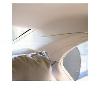
Take out the loudspeaker cover 2, and where necessary remove the loudspeaker underneath
