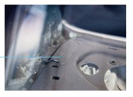
Using a suitable tool, carefully cut into the insulation underneath (5) at the edge of the parcel shelf along the markings shown and/ or carefully cut into the pre-existing perforations on the component and fold back, paying attention to the electrical wires
