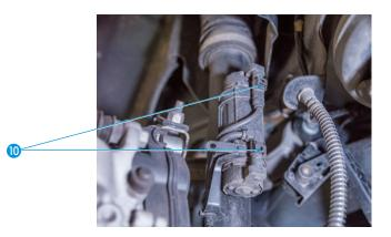
• Disconnect the screw connection (1) on the transverse link and dismount the transverse link
