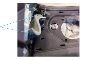
Pull the air suspension module downwards and remove
