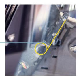
Use the lifting platform positioning points as stipulated by the vehicle manufacturer. Risk of death from vehicle slippage.
