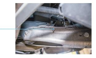
Disconnect the air suspension module's connecting wire (1) and decouple it from the bracket
