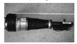
■ Fit new strut upwards and position the 3 upper nuts ⑧.
