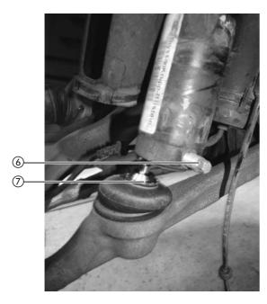
■ Push the bottom track control arm down and remove the strut sideways and downwards.
