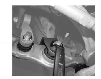
■ Remove the strut bottom fixing fork ⑦.
