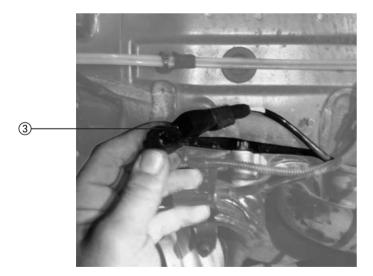
Insert plug (shock absorber valve) of the strut being fitted ③.
