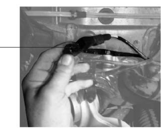
■ Remove plug (shock absorber valve) of the strut being dismantled ③.
