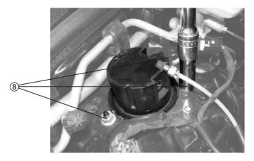
■ Fit new strut upwards and position the upper nuts ⑧.
