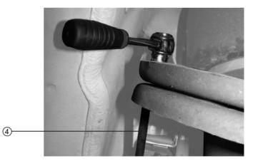
Dismantle level sensor linkage ④.
