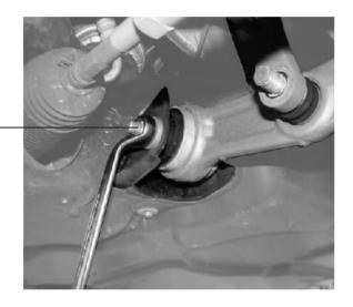
■ Loosen the inner fixture of the bottom track control arm ⑥.
