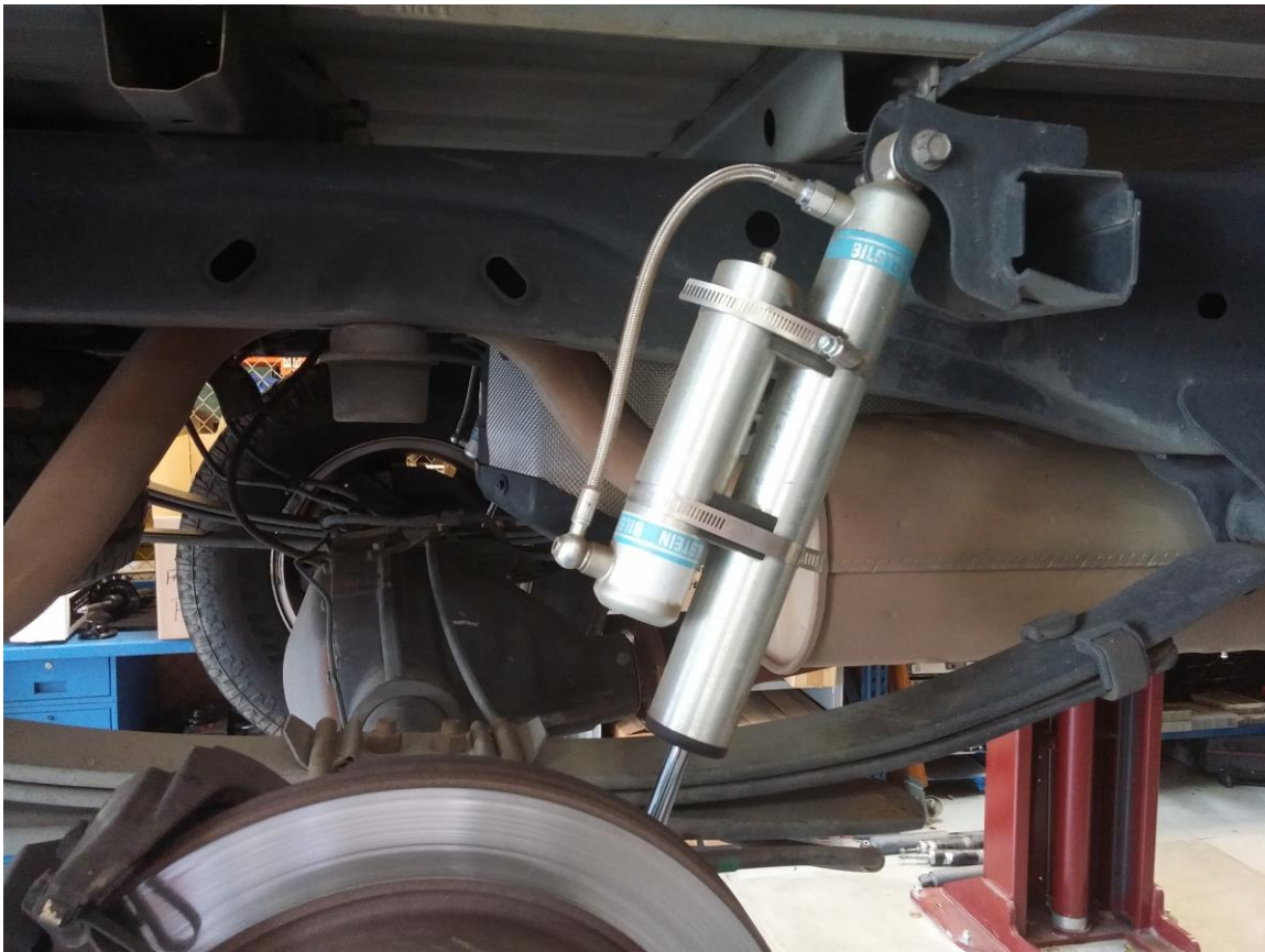
Figure 1. Reservoir placement for both sides
