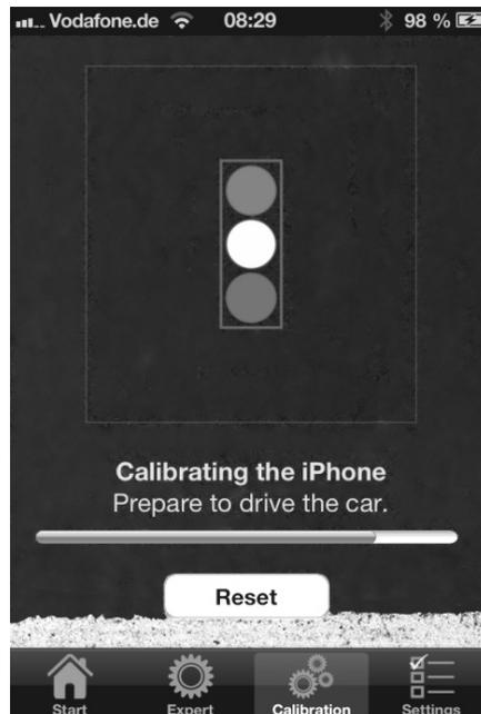
For full functionality of your BILSTEIN iRC you can calibrate the system in the Calibration screen to inform the BILSTEIN iRC about the directions of the longitudinal and lateral axis of the vehicle. The calibration will be saved in the control unit and must be done only once.
