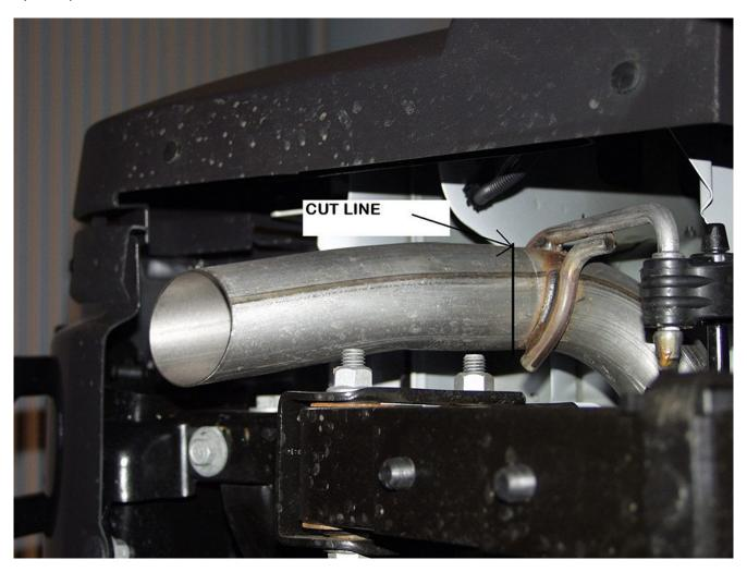
4) At the front of the muffler, cut just in front of the weld. (see picture)
