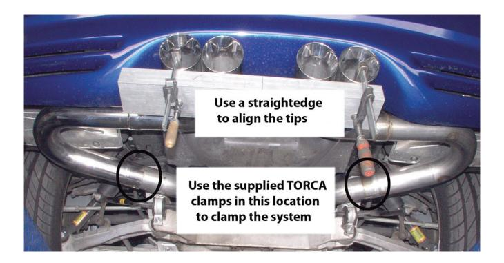
8. With all components in place, use a straight edge along the bottom of the tips for proper alignment. The tips are designed to follow the curve at the rear facia, so they may angle out slightly. Keep in mind that it may take some time to align them correctly.
