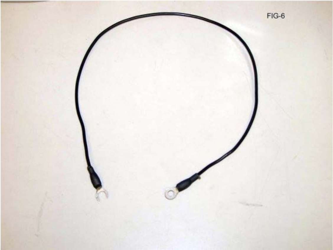
Route ground extension wire behind right side kick panel up towards the bottom of the dash, loosen bolt shown (Figure 7) and install open end connector and tighten.
