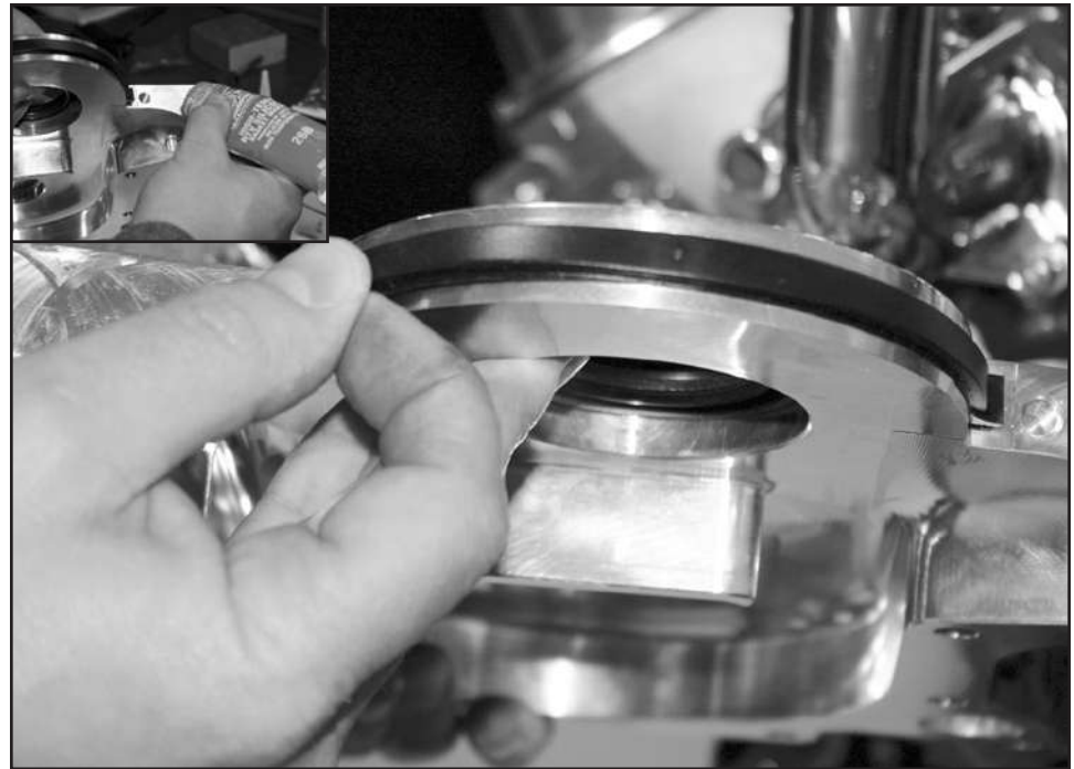
Figure 4: Prepare Timing Cover For Installation
