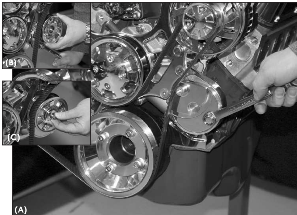
Figure 22: Install Tensioner Pulley & Serpentine Belt
