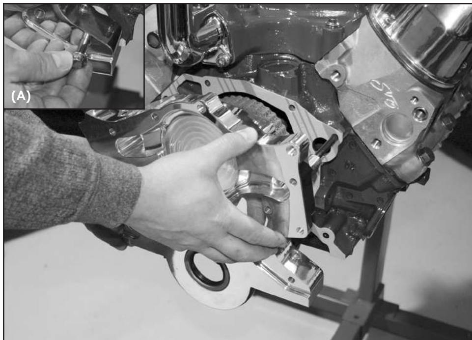
Figure 5: Install Timing Cover & Gasket
