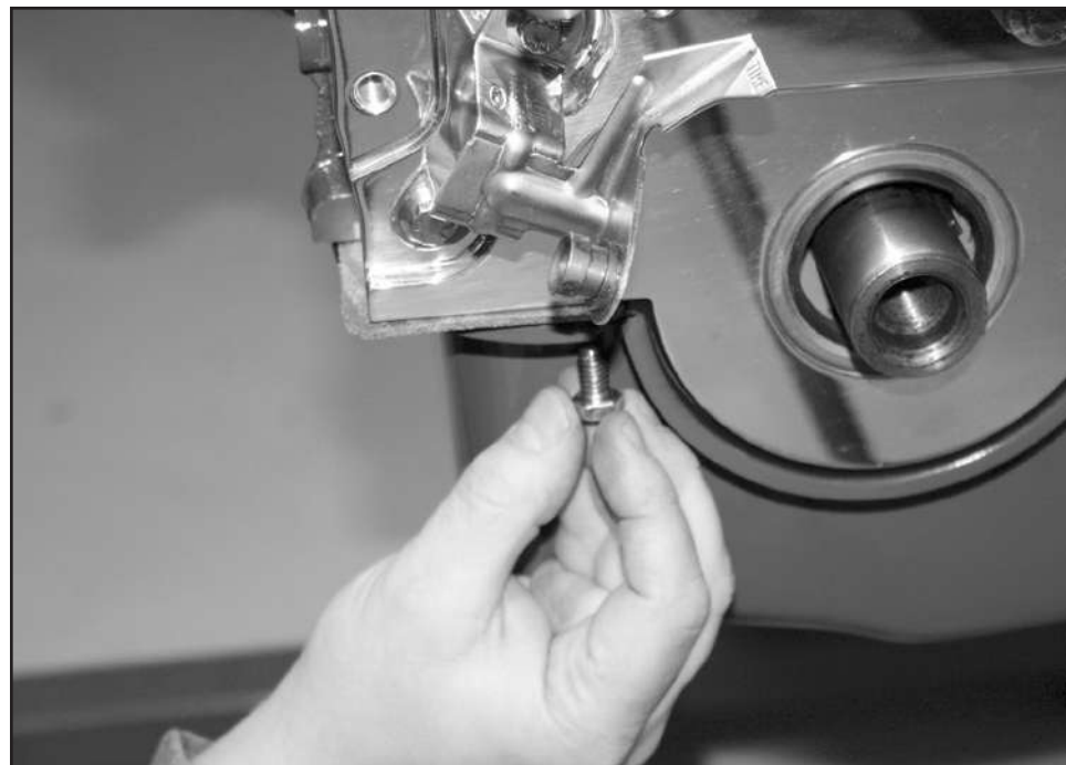
Figure 10: Oil Pan Installation (If Removed)
