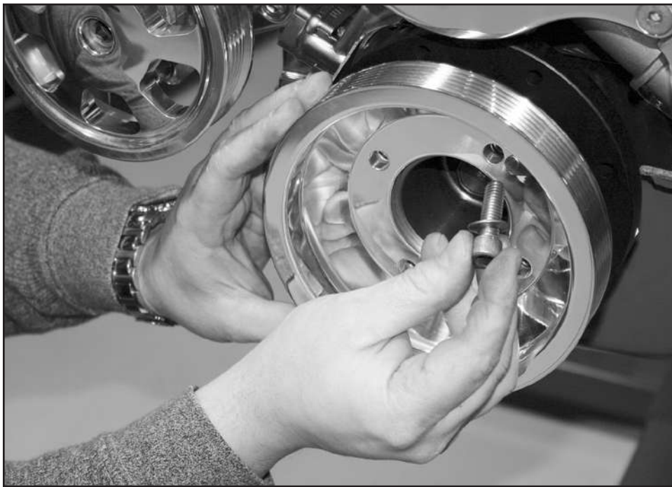
Figure 19: Install Crankshaft Pulley
