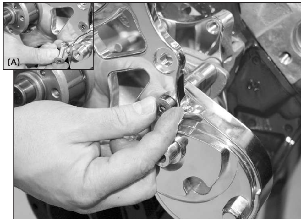
Figure 16: Install Bridge Bracket (Continued)
