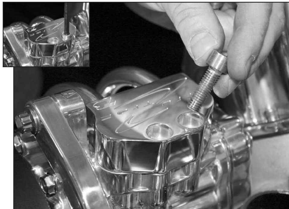
Figure 23: Install Compressor Manifold
