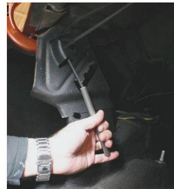
Figure A Torque Rod Removal
