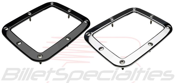
Billet Specialties Smooth Shifter Boot rings offer a clean look to match any interior. Shifter boot rings are precision machined from 6061-T6 Aluminum and available in either a polished or black anodized finish. Includes stainless self- tapping hardware and fits leather or rubber shift boots.
