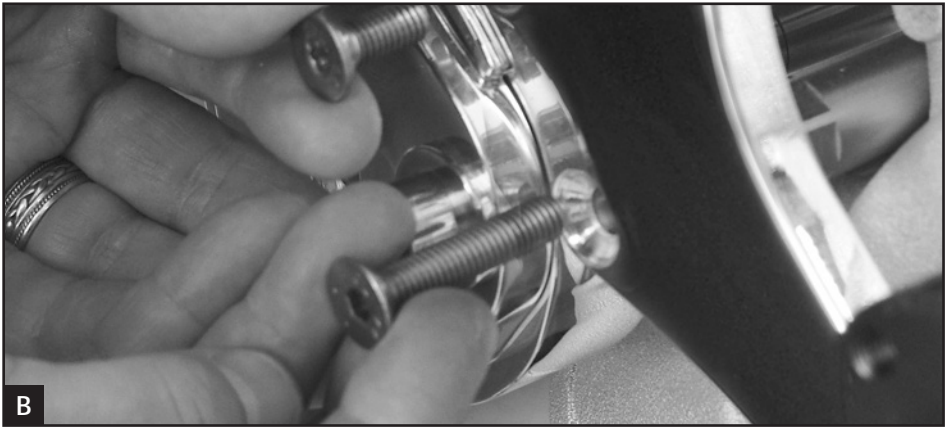
Figure 7: Attaching Bridge Bracket
