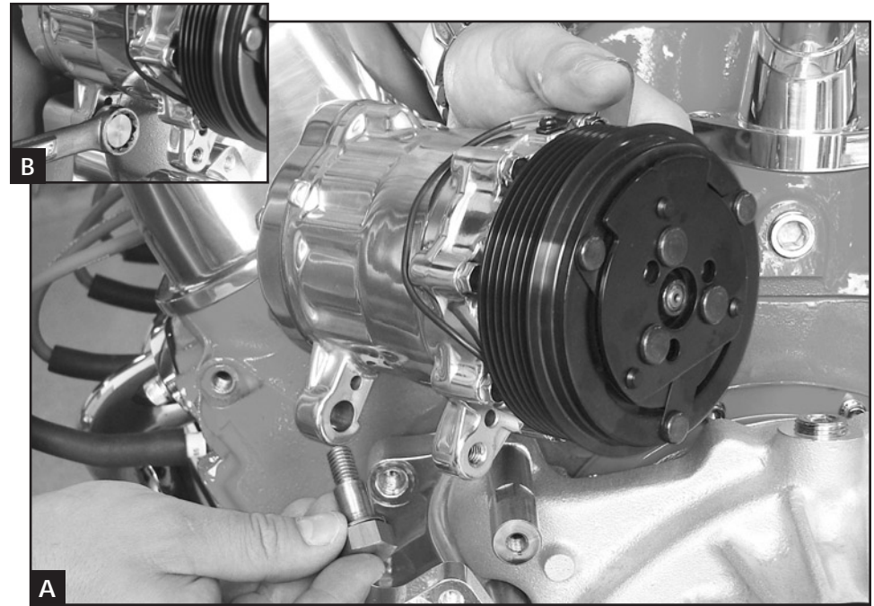
Figure 8: Install SD-7 Compressor
