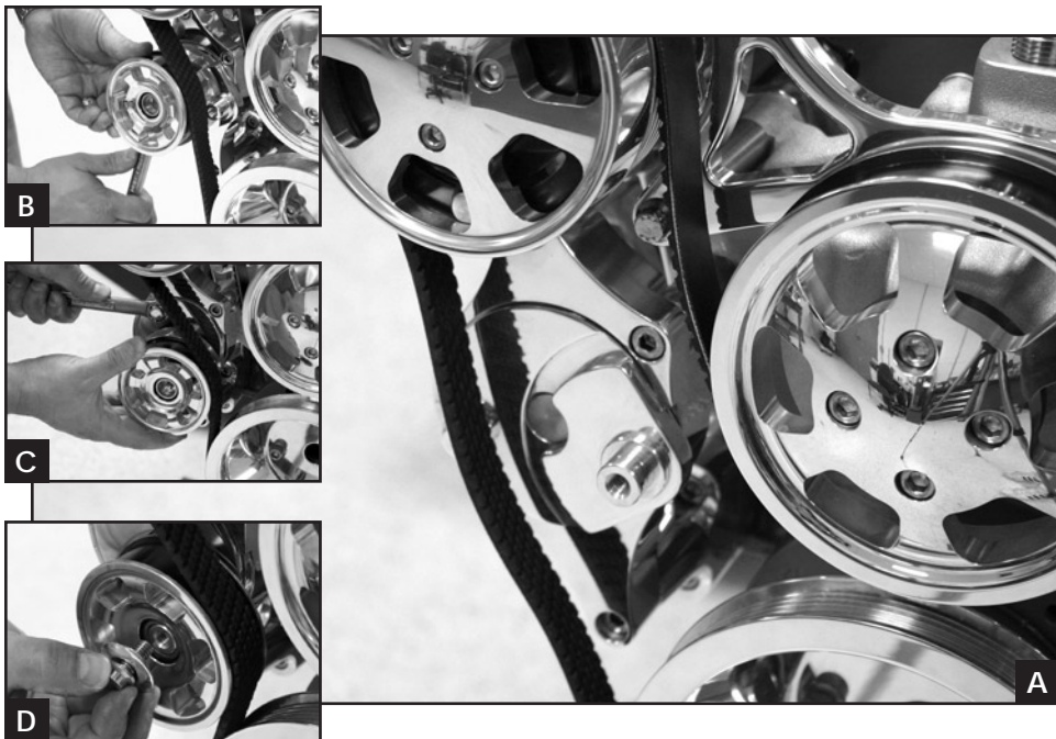
Figure 14: Install Serpentine Belt & Tensioner Pulley
