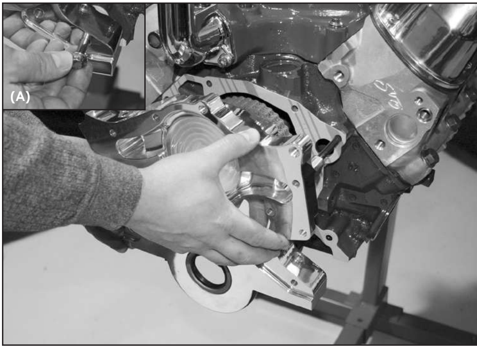
Figure 5: Install Timing Cover & Gasket
