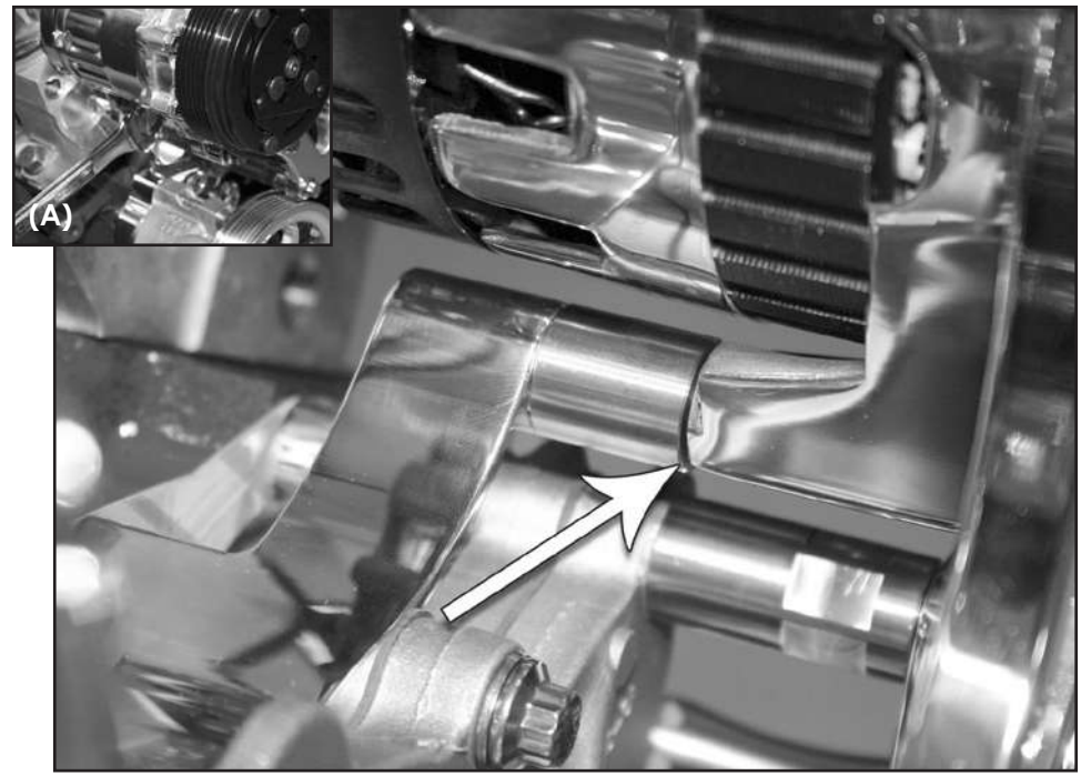
Figure 18: Complete Bridge Bracket Installation
