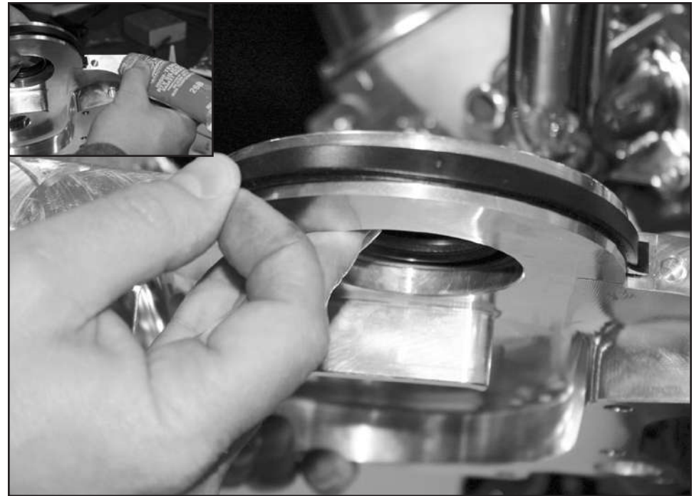
Figure 4: Prepare Timing Cover For Installation
