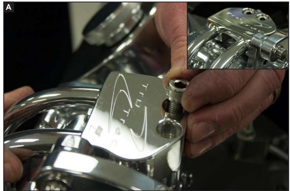
Figure 14: Install Compressor Manifold
