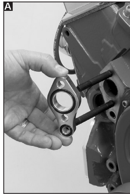
Figure 2: Install Water Pump Spacer & Alternator Bracket
