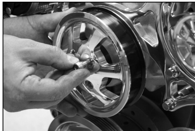
Figure 12: Install Water Pump Pulley
