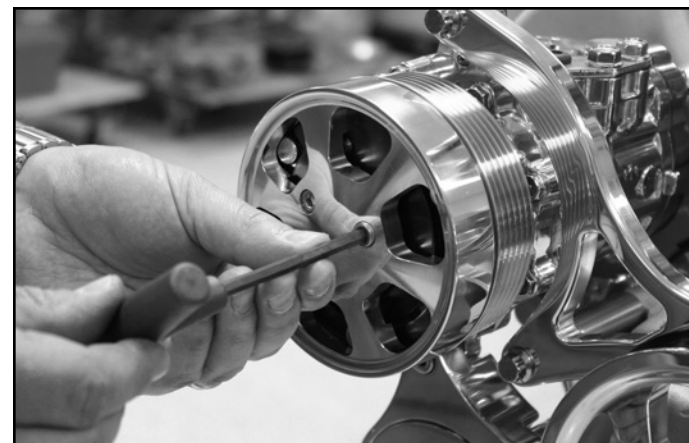
Figure 13: Install Compressor Clutch Cover
