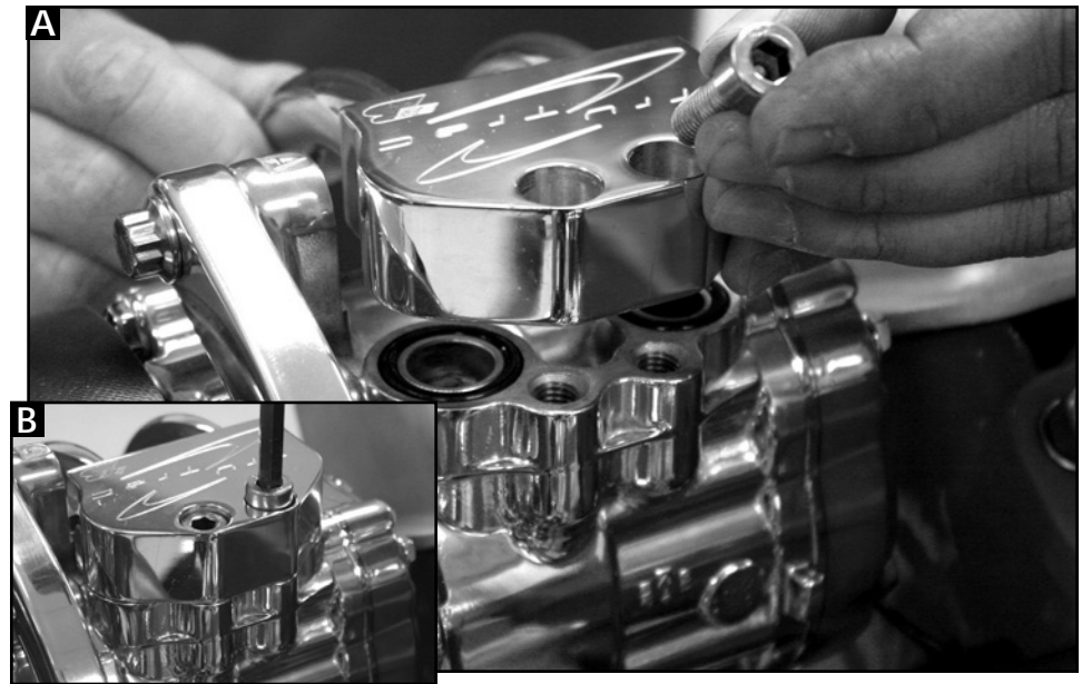
Figure 15: Install Compressor Manifold
