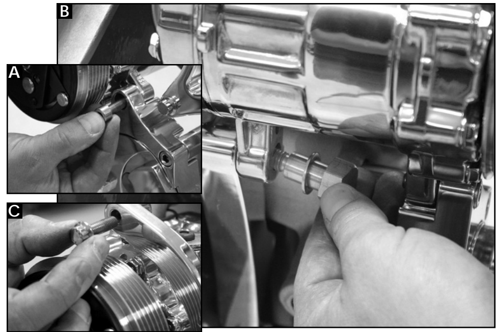
Figure 10: Install A/C Compressor
