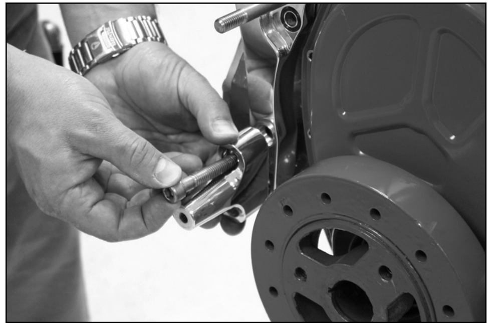
Figure 4: Install Tensioner Support Bracket
