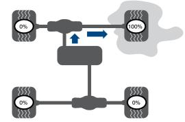
LOCKING OF THE CENTRE DIFFERENTIAL: 50% of the torgue goes to the rear wheels. The vehicle progresses.
