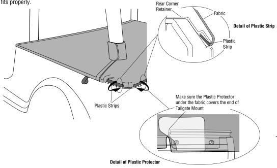
Note: The Plastic Protector sewn into the fabric must be located over the Tailgate Retainer Mounts.
