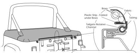
**Note:** The Plastic Strip on the bottom of the cover will not be used and wide tucked up under the bows.
