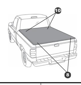
Driving with the Tonneau Open 9 Fold Tonneau Forward Fold the Tonneau toward the front of the vehicle.
