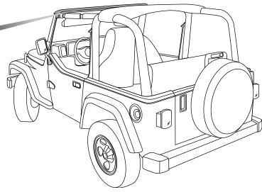
**Note:** While installing the Windshield Retainer/J-Hook Bracket Assembly, apply firm pressure toward the front of the vehicle to make sure that the assembly is installed correctly over the bulb seal.
